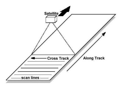
**Figure 2-3:** Schematic of a MODIS Observation Swath.
