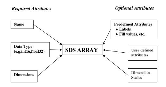
**Figure 2-1:** Schematic of the Required and Optional Components (Attributes) of an SDS The required components are shown on the left side of the figure, and the optional components are shown on the right.
