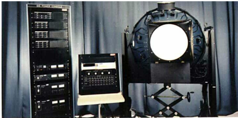
Figure 12: MODIS reflective solar bands pre-launch calibration source: SIS-100
