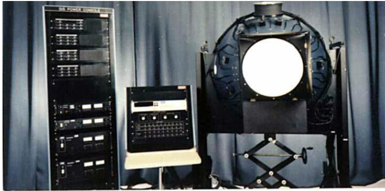
Figure 13: MODIS reflective solar bands pre-launch calibration source: SIS-100
