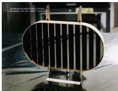
Figure 7: On-Board Blackbody Calibration Source
